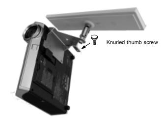
C. After completing the service procedure swing the projector back up and re-install the knurled thumb screw.
